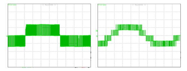
In order to achieve the three-level output, the output section has to have twice the number of output switches plus clamping diodes as shown below. The benefit gained by using a three-level output is reduction in voltage amplification at the motor due to reflected wave, lower common mode voltage, shaft voltage, and bearing current.
